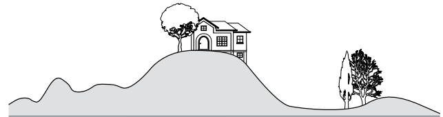
REGION A - N4 (W50) REGION B - N5 (W60) AND REGION C - C4 (W70) EXTREMELY SEVERE - ISOLATED BUILDING ON THE CREST OF A HILL
