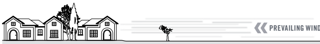
REGION A - N2 (W33), REGION B - N3 (W41) AND REGION C - C2 (W50) STRUCTURES BUILT ADJACENT TO AN OVAL OR LARGE VACANT LOT SUBJECT TO PREVAILING WINDS.
