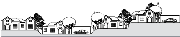
REGION A - N2 (W33), REGION B - N3 (W41) AND REGION C - C2 (W50) STRUCTURES ON UNDULATING TERRAIN IN SUBURBIA
