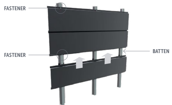
Figure 7.0: Shadowline Gap Range Between Panels
